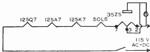
Fig. 1. The filament circuit of a typical a.c.-d.c. receiver.
